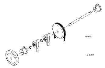
Clean the shaft and slide the pillow block bearings off of the shaft.
